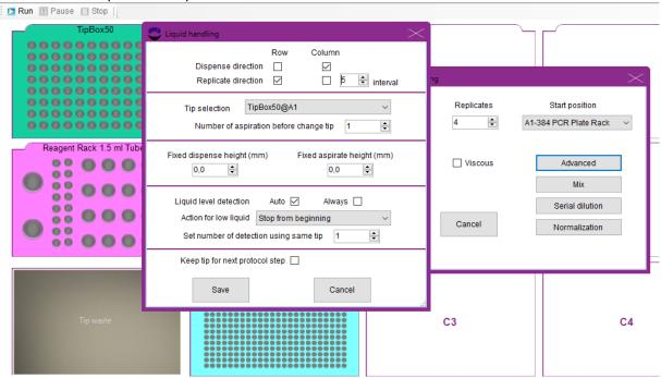
Sample in well A1 is now dispensed in wells A1, A7, A13 and A19. Sample in well B1 is now dispensed in wells B1, B7, B13 and B19.
