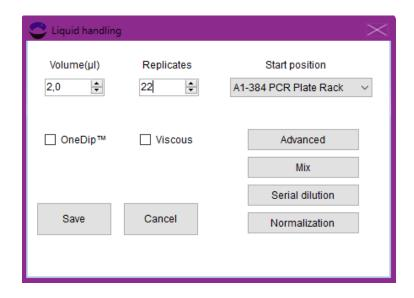
3. Open Advanced menu. Set Replicate direction to row, see screen capture below. Save the protocol step. Set-up is ready.
