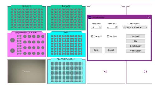
5. Open the "Advanced" menu. Set Replicate direction to row and interval to 5, see screen capture below. Save the protocol step.
