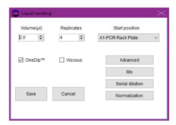
5. Mark the fw primers and drag them to the PCR plate to open the liquid handling window. Set volume to 2 and replicates to 8, see screenshot below. Do <u>not</u> use OneDip™ because of possible contamination issues.
