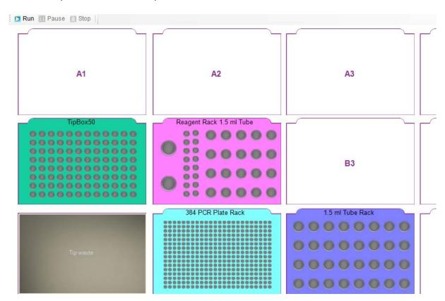
2. Create a partial 384 plate by marking wells A1 to K16 and then use a right click and select Dispense pattern. Screen capture below shows how the plate looks like.
