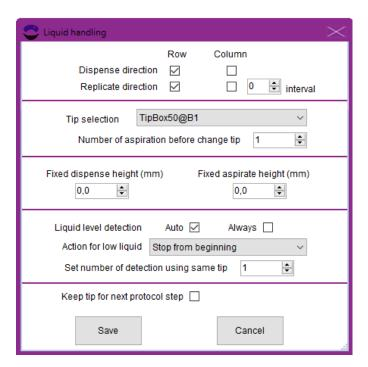
4. Mark sample plus NTC water tubes and drag them to the 384 plate to open the liquid handling window. Set volume to  $\geq 2 \mu l$ , replicates to 2 and select OneDip<sup>TM</sup>, see screen capture below.
