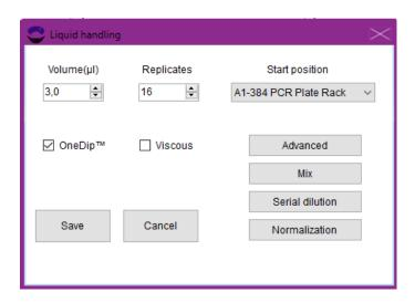
3. Open Advanced menu. Set both Dispense and Replicate direction to row, see screen capture below. Save the protocol step.
