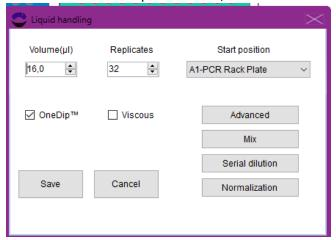
4. Mark the fw primers and drag them to the PCR plate to open the liquid handling window. Set volume to 2, replicates to 4 and select OneDip™ in order to save time and tips, see screenshot below. Always start to dispense the primer type (forward/ reverse) that have more variants, in this case fw primer. This will save tips and time.
