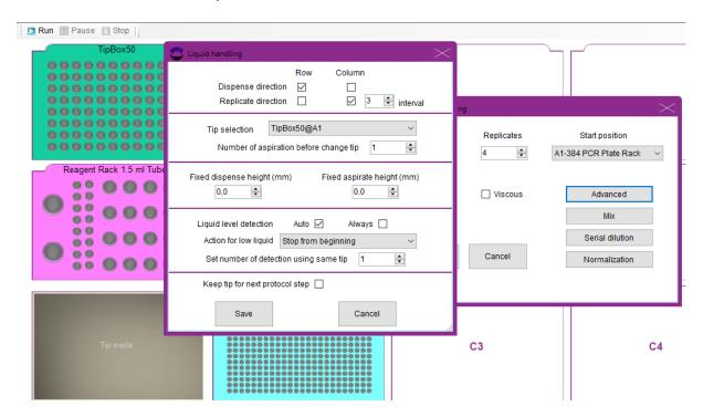
Sample in well A1 is now dispensed in wells A1, E1, I1 and M1. Sample in well B1 is now dispensed in wells A2, E2, I2 and M2.
