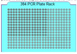
2. Mark the 13 tubes containing the gene mixes and drag them to the 384 plate to open the Liquid handling window. Set volume to  $\geq$ 3  $\mu$ l, replicates to 16 ((No samples x No of replicates) + No of NTC's) and select OneDip, see screen capture below.
